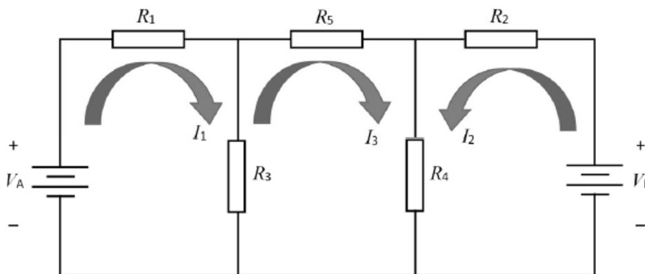
$$R_3I_1 = R_4I_2 + (R_3 + R_4 + R_5)(I_3)$$
