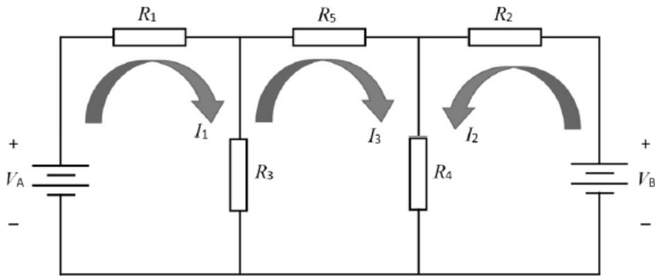
$$62-R_3I_1 = R_4I_2 + (R_3 + R_4 + R_5)(I_3)$$
