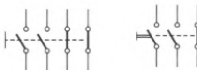
FIGURA 8 – CONTATOS (2NA + 2NF) E (1NA TRAVA + 1NA + 1NF).
