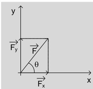
$$\begin{aligned} \text{sen } \beta &= \frac{F_y}{F} \Rightarrow F_y = F \text{sen } \beta \\ \text{cos } \beta &= \frac{F_x}{F} \Rightarrow F_x = F \text{cos } \beta \end{aligned}$$
