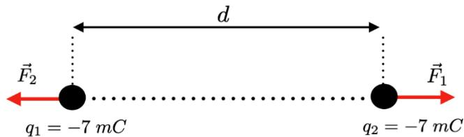
$$\begin{aligned} |\vec{F}'| &= k_0 \frac{|q_1||q_2|}{d^2} \\ &= (9 \cdot 10^9) \times \frac{(7 \cdot 10^{-3})^2}{(171,46 \cdot 10^3)^2} \\ &= 1,5 \cdot 10^{-5} \text{ N} = 15 \cdot 10^{-6} \text{ N} = 15 \mu\text{C} \end{aligned}$$
